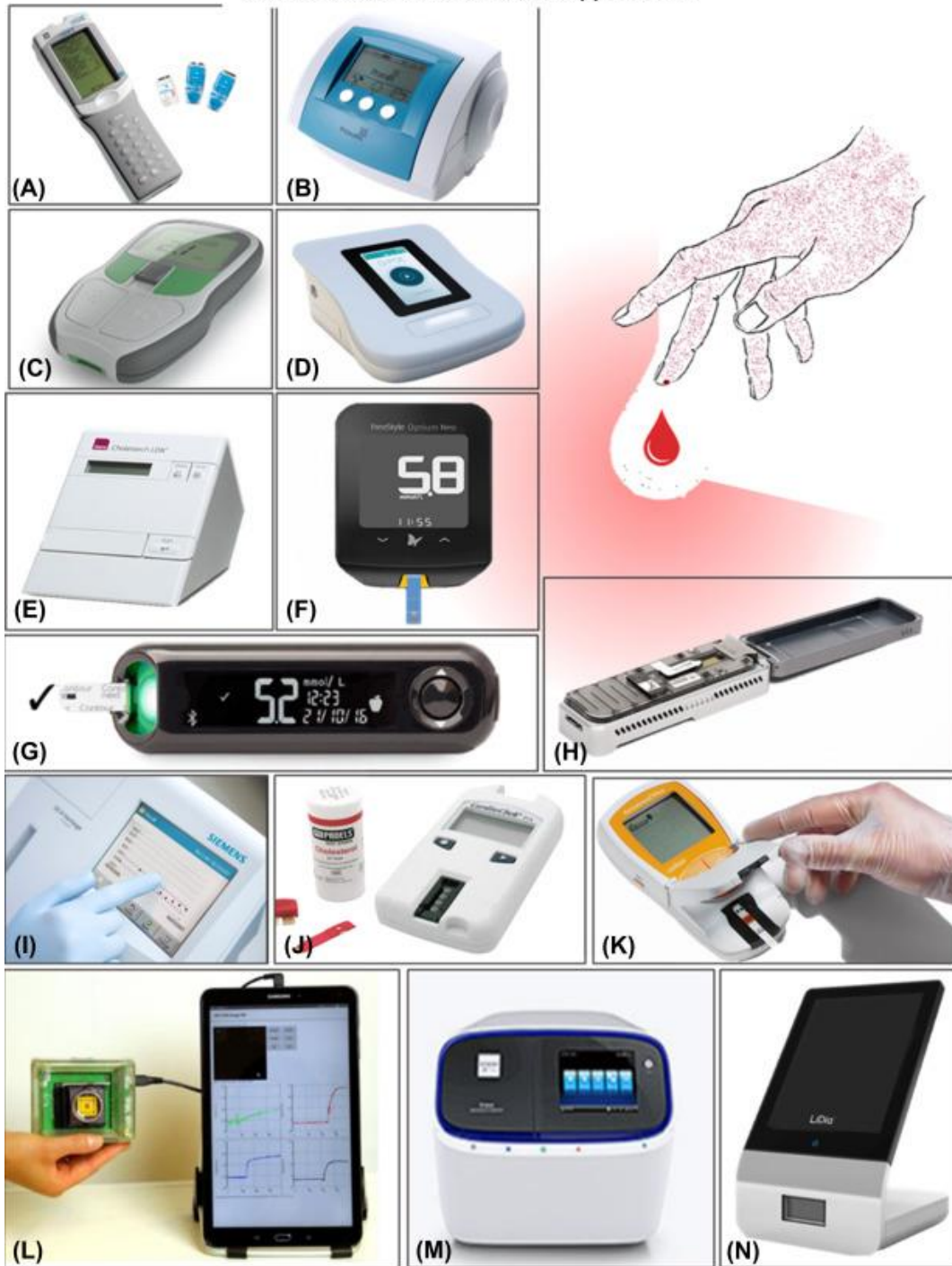
Figure 9 Demonstrations of some commercialized POC biosensors. Most of them are conventional design containing a measuring device and a disposable testing strip. Figure reproduced from [117,128].
