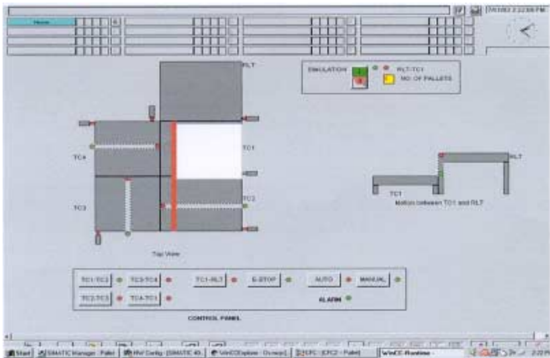
Figure 12. Motion of pallet from TC1 to TC2 table
