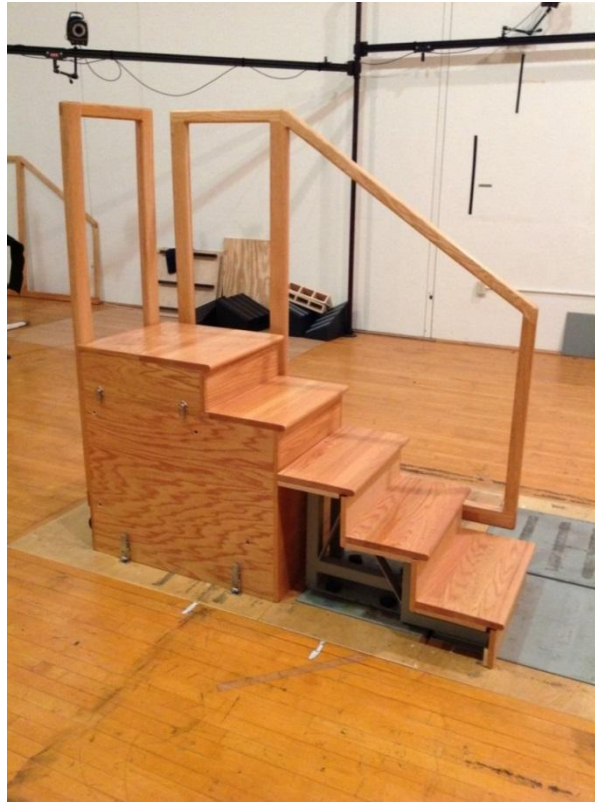
Figure 6. Complete setup of 5-step staircase for experimental data collections
