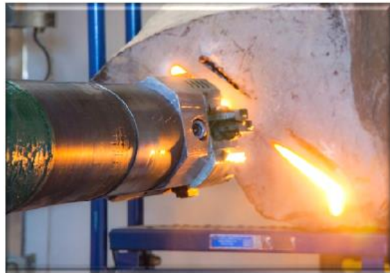
Figure 9. Laser Mechanical Drill Bit [28]
