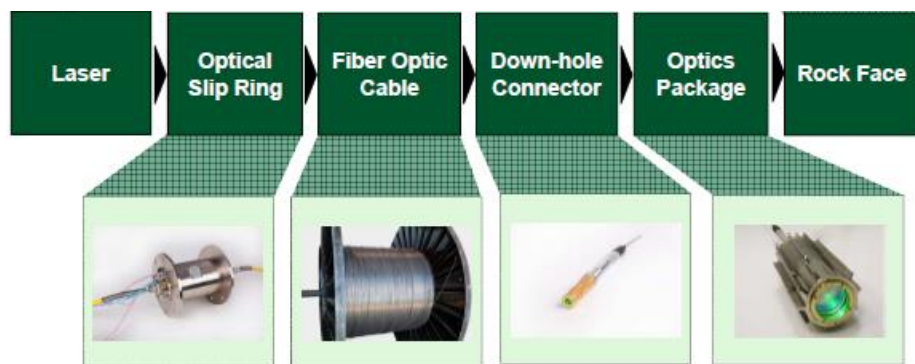
Figure 10. Laser Power Transmission Process [28]
