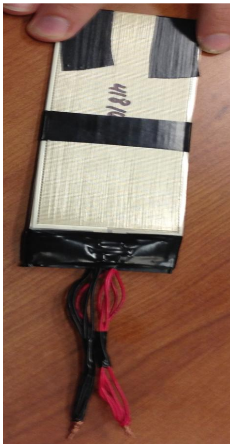
Figure 10. Six PFC-W54 Strips with Leads Pre-Attached
