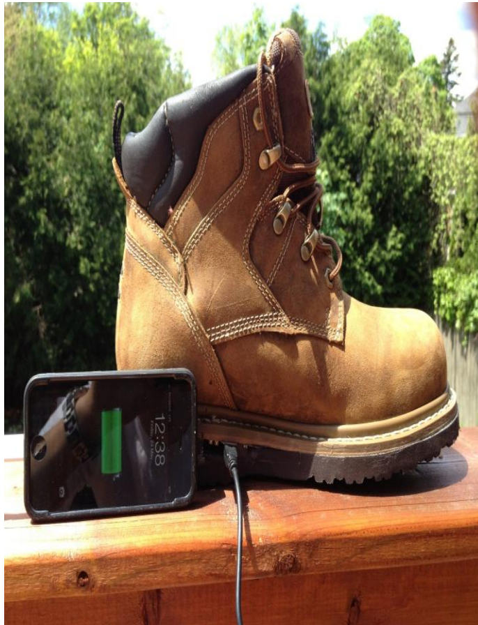
Figure 2. PowerSole uses a Faraday Coil to Charge a Battery
