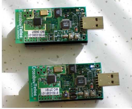
Figure 3-3: Crossbow/UC-Berkeley’s TelosB sensor platform
