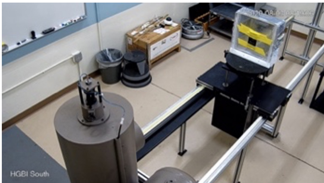
Figure 4.1: Irradiation of a Samsung Galaxy S9 mounted on a PMMA slab phantom using a ^{137}\text{Cs} source at LANL.
