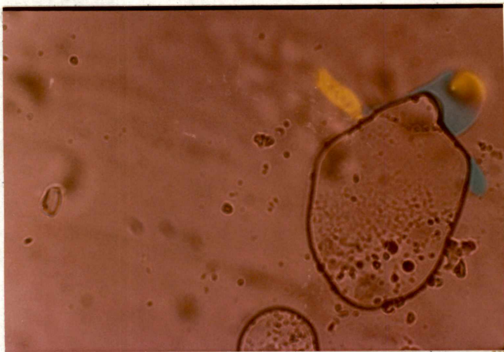
Figure 29. The "D" phase, " M_1 " phase, "viscous isotropic," "G" phase and "A" phase in dodecyl amine - ND_2/D_2O system disappear. Crossed polars \leftrightarrow , x200.
