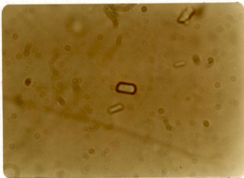
Figure 6. Three-dimensional hexagonal single crystal phase or "A" phase in dodecyl amine \text{-NH}_2 /water system 0% weight water, showing no parallel layer structure. Crossed polars \leftarrow \updownarrow \rightarrow , x1000.
