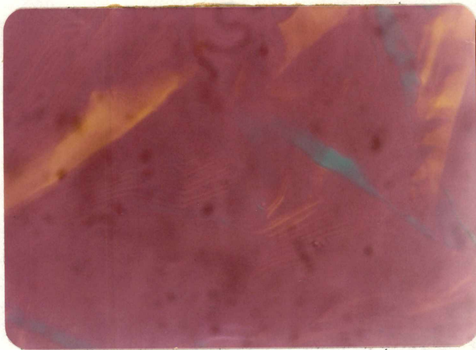
a. The "neat" phase structure in dodecyl amine -NH 2 /water system 70% weight water. Crossed polars \leftrightarrow , x1500.
