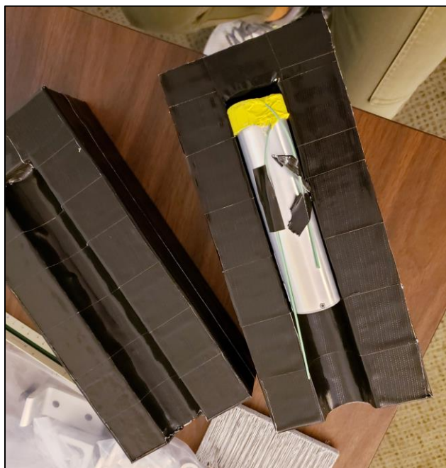
Figure 25. A 3D-printed shield designed with CZT dimensions for use in fume hood (CZT and sample loop also pictured).
