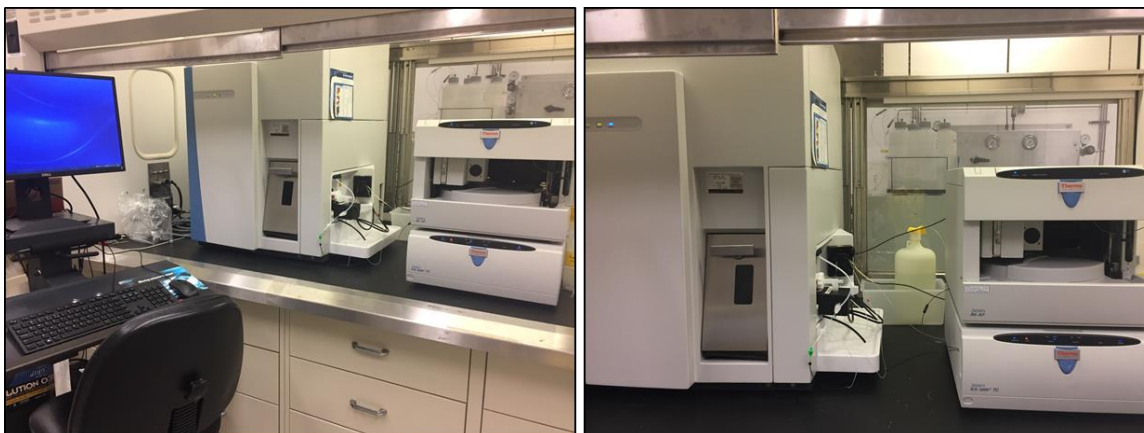
Figure 23. Photos of the original coupled HPIC-ICPMS system in a radiological fume hood.
