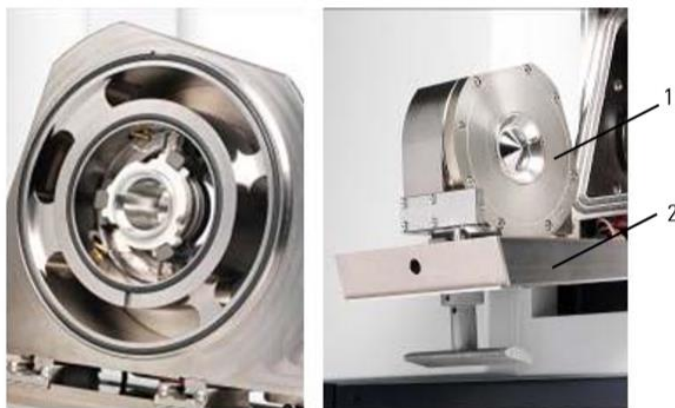
Figure 15. Right: the interface block (1) and the plasma door (2). Left: a view of the extraction lens, located behind the cones (side not shown on the right) 181 .
