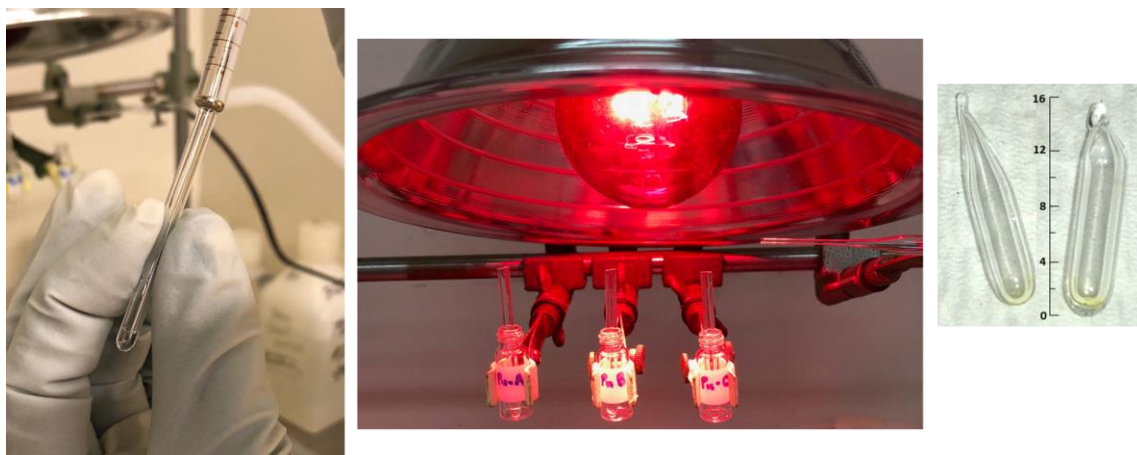
Figure 30. Ampoule filled via syringe (left), solution dried by heat lamp and air flow (middle), final sealed targets of certified reference standard U930-D (93.2% ^{235}\text{U} ) in high-purity silica ampoules 208 . Inset: scale in mm (right).
