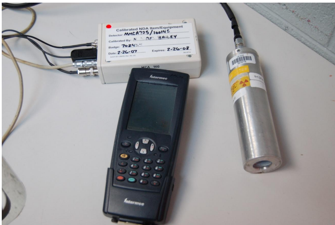
Figure 6: Example of typical NaI detection equipment including detector, multi-channel analyzer (MCA), and hand-held computer.
