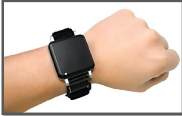
Figure 4. Positioning of the inertial movement unit (IMU) on the wrist.
