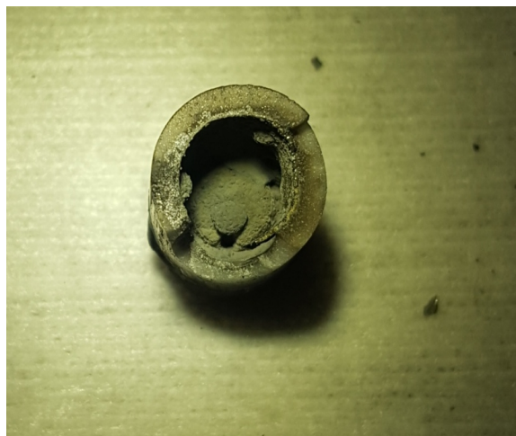
Figure 3.15: Heater (possible melt wires shown near bottom-center of crucible) after January 23, 2020 test.
