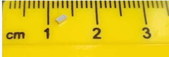
Figure 3.60: August 13, 2021 not melted Pt-Ir melt wire.
