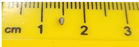
Figure 3.57: August 10, 2021 melted Pt-Ir melt wire.
