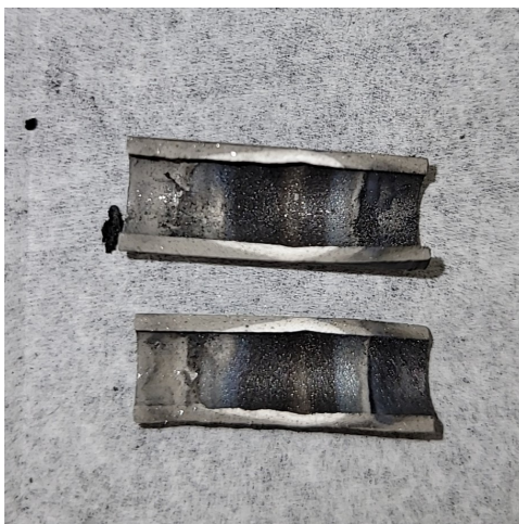
Figure 3.27: July 20, 2021 high purity MgO post-test observation of scorching within crucible.
