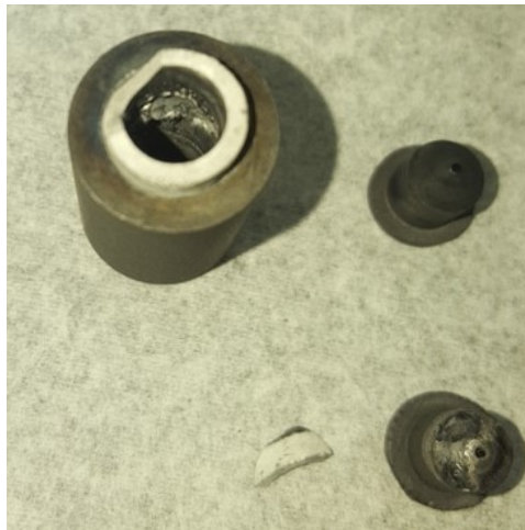
Figure 3.21: June 22, 2021 HfO_2 post-test observation of arcing effects within crucible.
