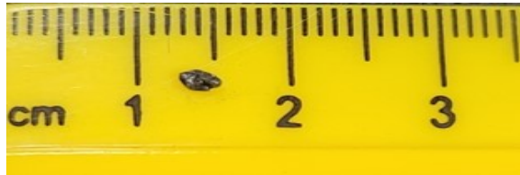
Figure 3.61: August 17, 2021 melted Pt-Ir melt wire.
