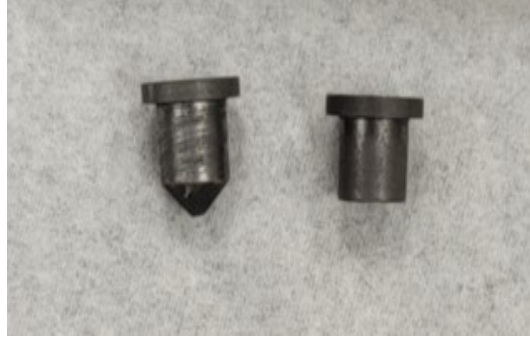
Figure 3.28: Comparison between tapered (left) and flat (right) heater plugs.
