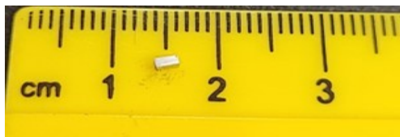
Figure 3.50: Unused and not melted Pt-Ir melt wire.
