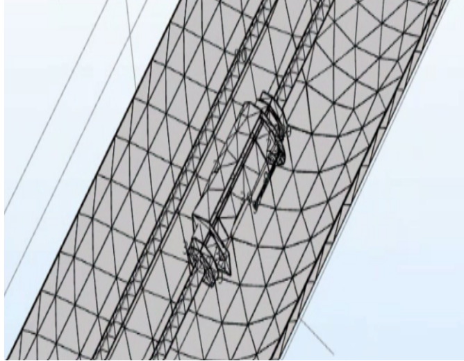
Figure A.21: Free tetrahedral mesh for RHT investigations with 12979 elements .
