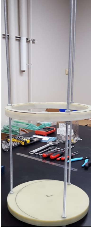
Figure 3.63: Frame of in-pile basket.
