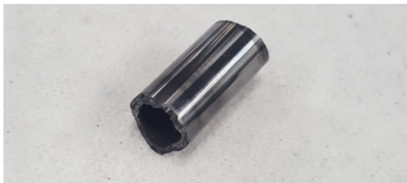
Figure 3.13: ZrO_2 that is no longer white following 1300 K test.
