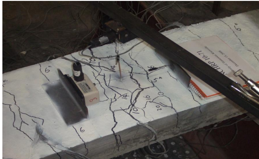
Figure 27: Flexural Crack Patterns at Failure (a) Specimen SB-1
