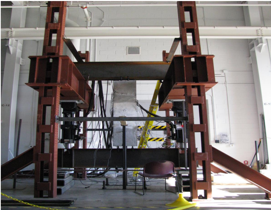
Figure 10: Tension Test Set-Up (Transverse Joint)
