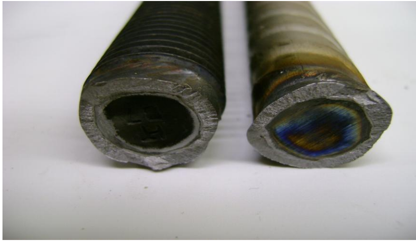
Figure 20: One Pass Weld Failure
