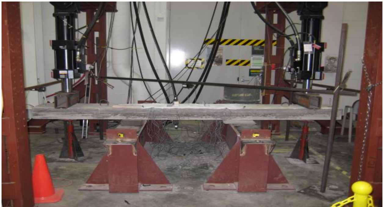
Figure 9: Flexural Test Set-Up (Longitudinal Joint Test)
