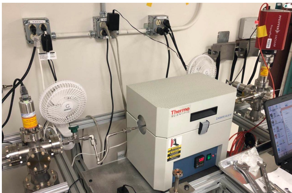
Figure 5.4 Gas driven permeation system for deuterium permeability in structural materials, or tungsten, analysis. Located in the Low Activation Materials Design and Analysis at Oak Ridge National Lab.
