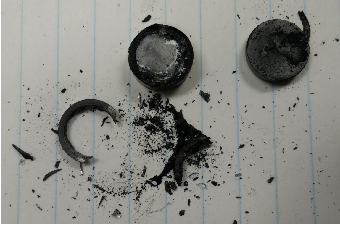
Figure 24 - The extracted graphite capsule and alumina powder compaction following the room temperature pressure test.
