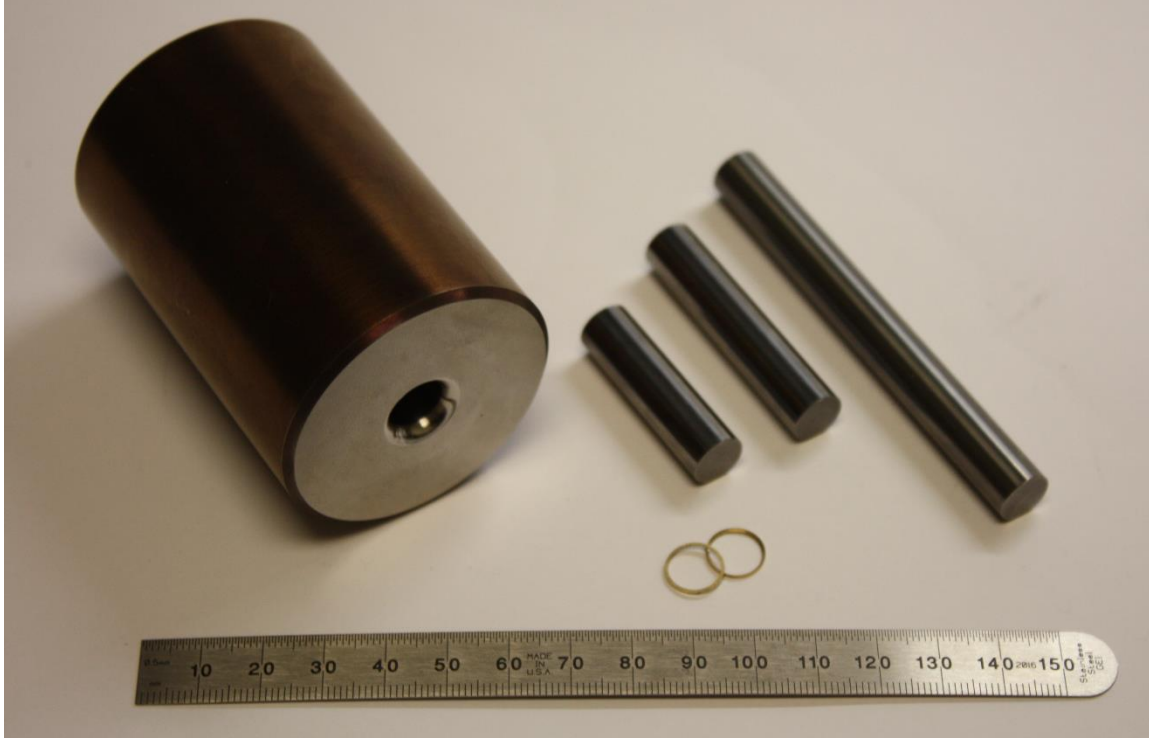
Figure 22 - The completed compaction cell, showing the fabricated cell body, tungsten carbide pistons, and anti-extrusions rings. The ruler in the foreground is in cm units.
