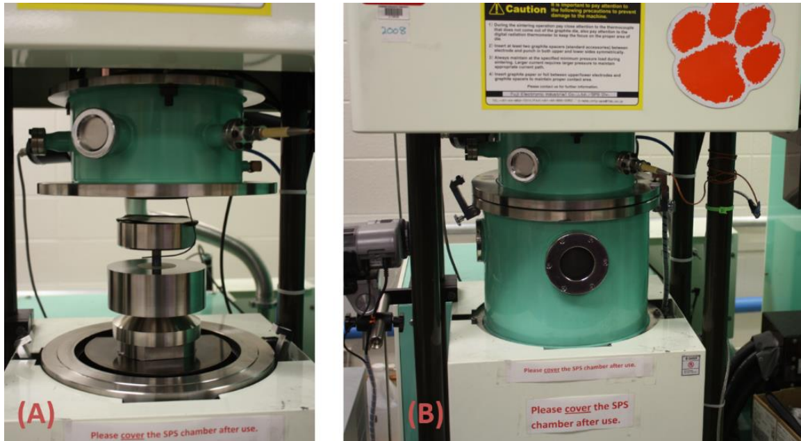
Figure 25 – The high pressure SPS cell undergoing testing at Clemson. In (A) the cell is visible before raising the vacuum chamber, and (B) the cell is enclosed and the vacuum pumped down.
