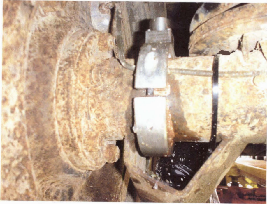
Figure 1.9: TSS/VSS accelerometer mounting location.
