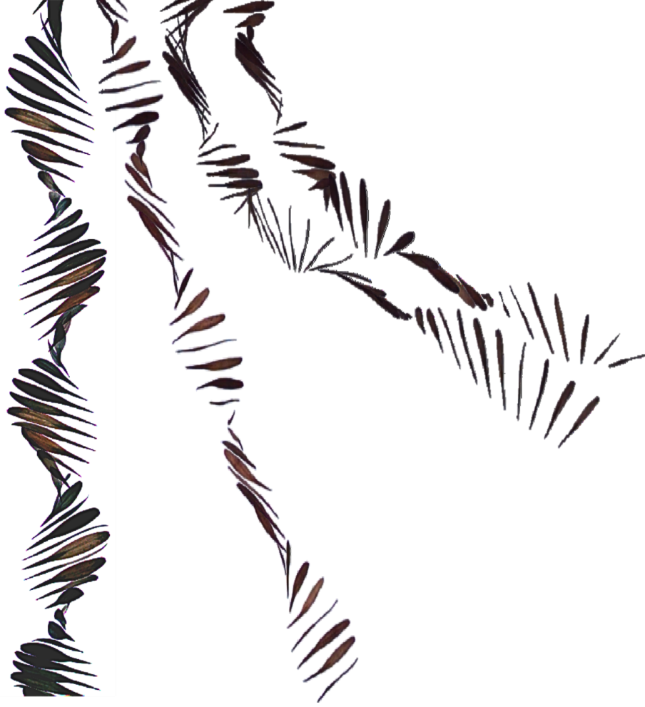
Figure 1.4: Time-resolved image sequences showing descent trajectories of F. Americana samaras under increasing crosswind speed. Each trace captures a stacked sequence of images extracted from high-speed video at 0.001-ms time intervals, illustrating spanwise rotation, precession, and lateral drift. From left to right: U = 0, 1, 3, 5 m/s.
