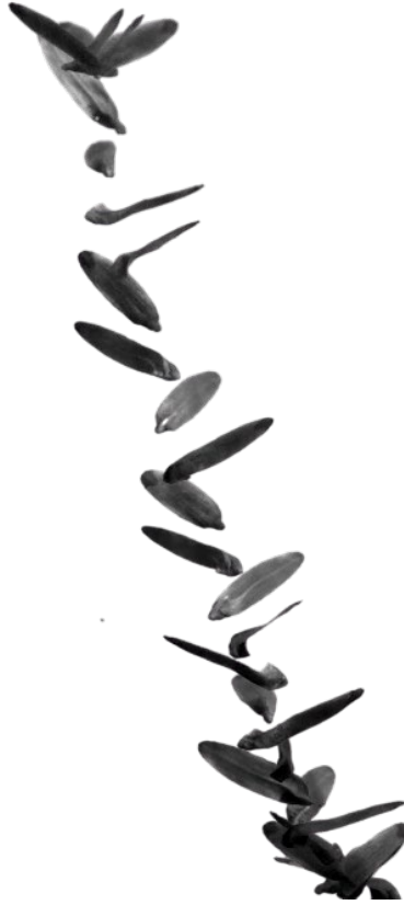
Figure C.1: Drop impact on the nutlet of a L. tulipifidera rolling samara illustrated with composite frames and tracked motion.
