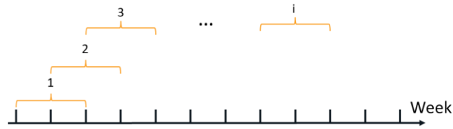
Figure 6.17. Illustration of the moving time window for input feature extraction.
