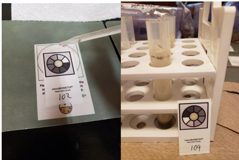
Figure 8: Soil microBIOMETER® test. Left: Drops being added to Soil microBIOMETER® grayscale card on provided green background. Right: Soil microBIOMETER® test tube with settled soil (Photos by Kara Grosso).
