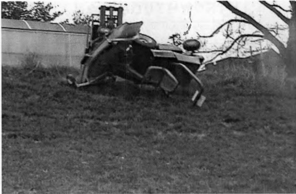
Figure 6-6. Measurement of yaw angle and slide distance on actual grass slope.
