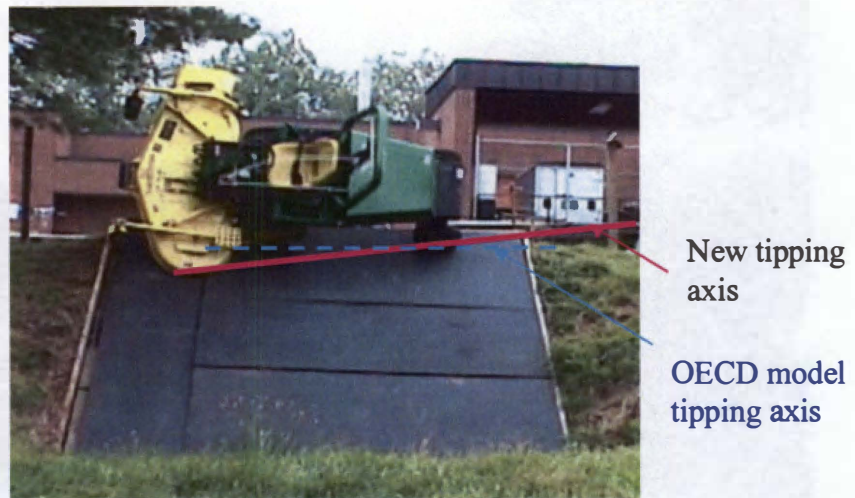
Figure 4-8. The axes change of rotation due to the deck size.
