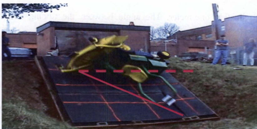
Figure 6-1. ROPS just hits the slope.
