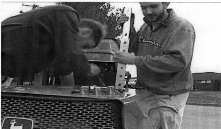
Figure 6-12. Mount the adjustable fitting for ROPS height extension to the mower frame.
