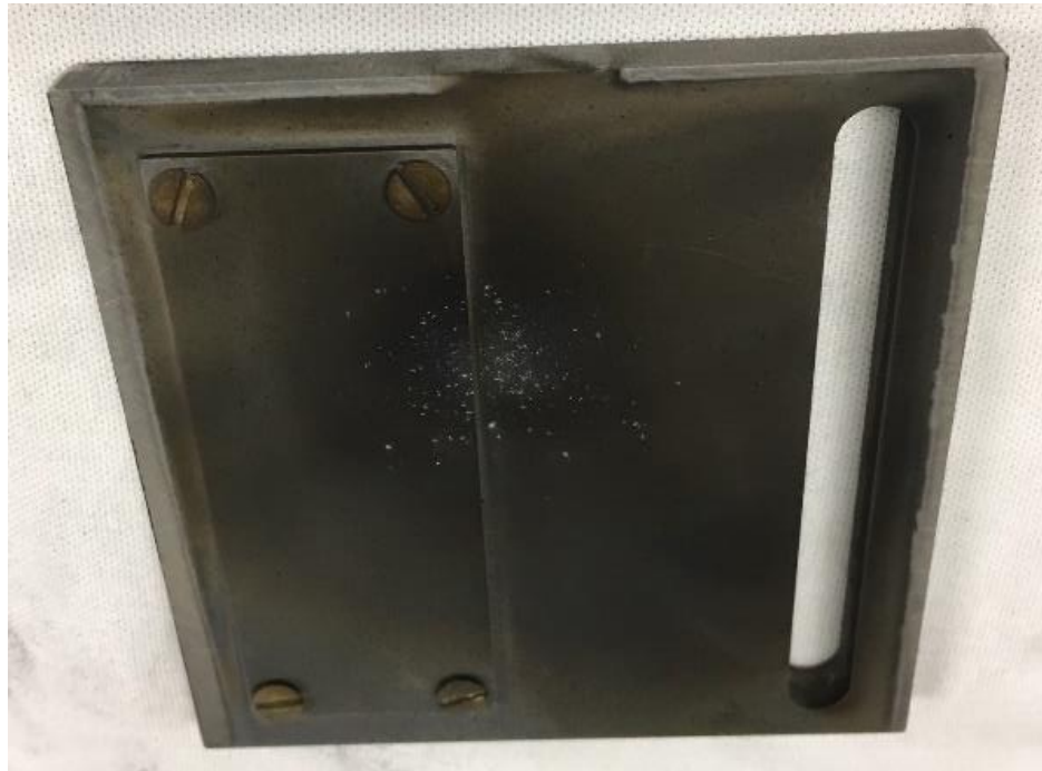
Figure 5.1. (a) ET-arc target pre-plasma exposure. Plasma impact on the target occurred at an angle of incidence 45^\circ above the cover the target to provide a small unaffected area adjacent to the plasma strike zone. (b) ET-arc target post-exposure.
