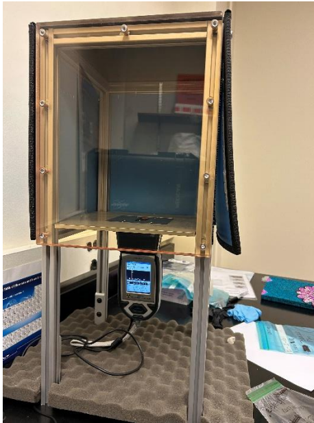
Figure 3.2: pXRF analyzer placed in a cubicle
