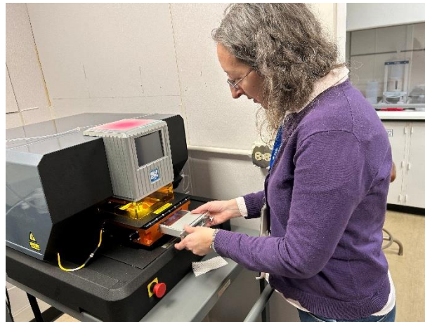
Figure 3.6: The laser cell being inserted into the laser chamber.
