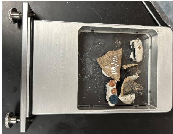
Figure 3.5: Pipe samples arranged in the laser cell.
