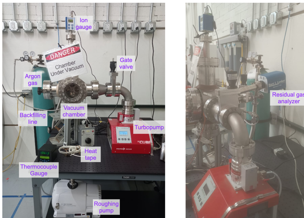
Figure 7.3: Left: front view of the upgraded vacuum chamber optimized for outgassing measurement. Right: side view of chamber; residual gas analyzer is connected at the back of the vessel. Credit: Sean Hollander and Chang-Hong Yu.
