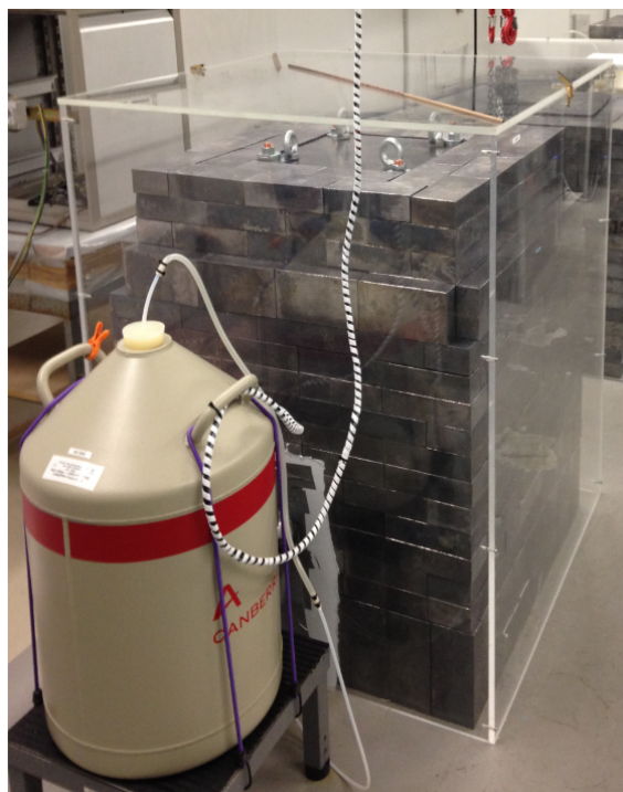
Figure 8.3: Gamma-ray spectrometer inside the Canfranc Underground Laboratory. Credit [63].
