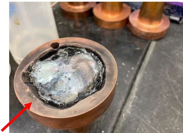
Crucible Melt Damage
