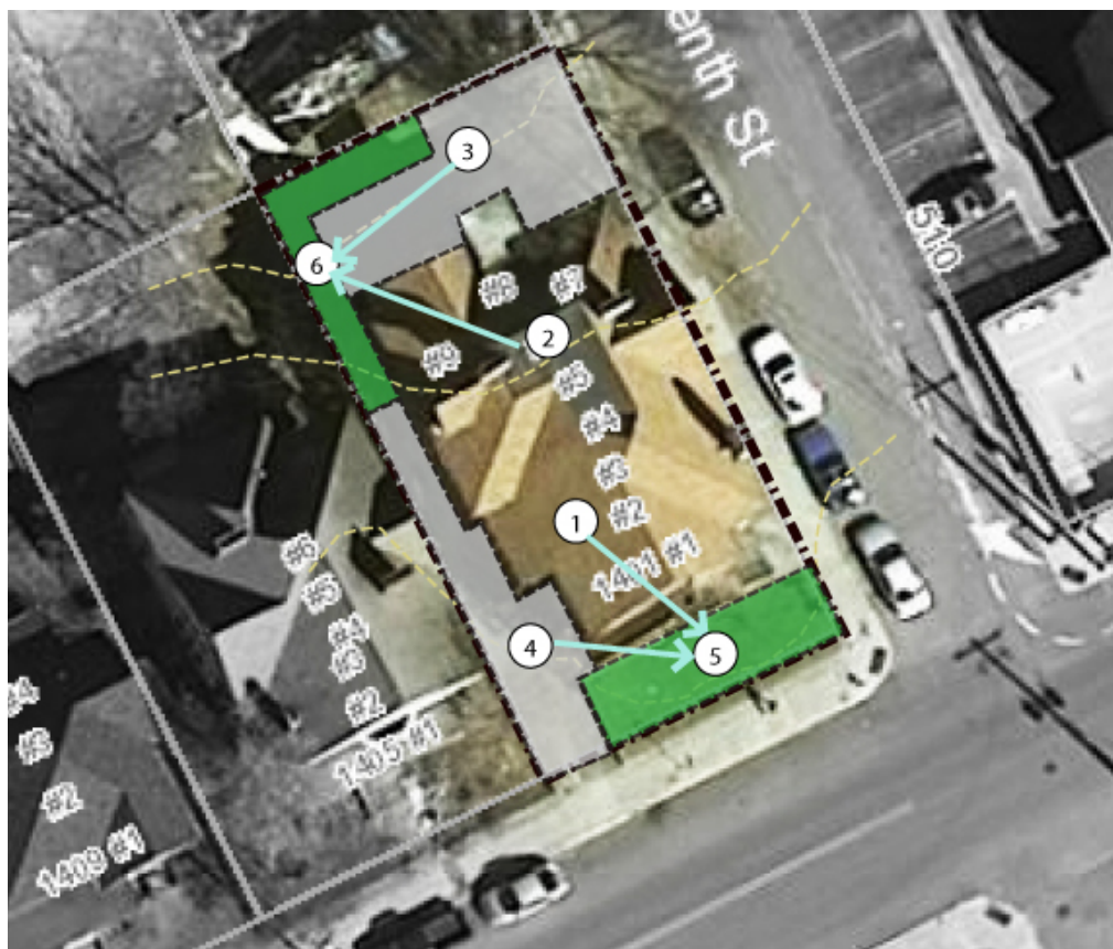
Figure 12: Runoff flow path inside the site
