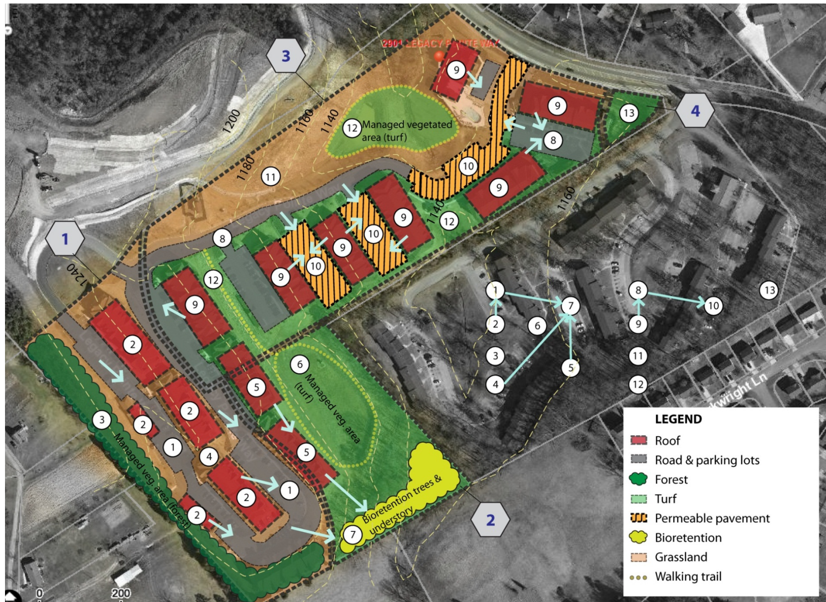
Figure 25: Placement of selected SCMs for the apartment complex project
