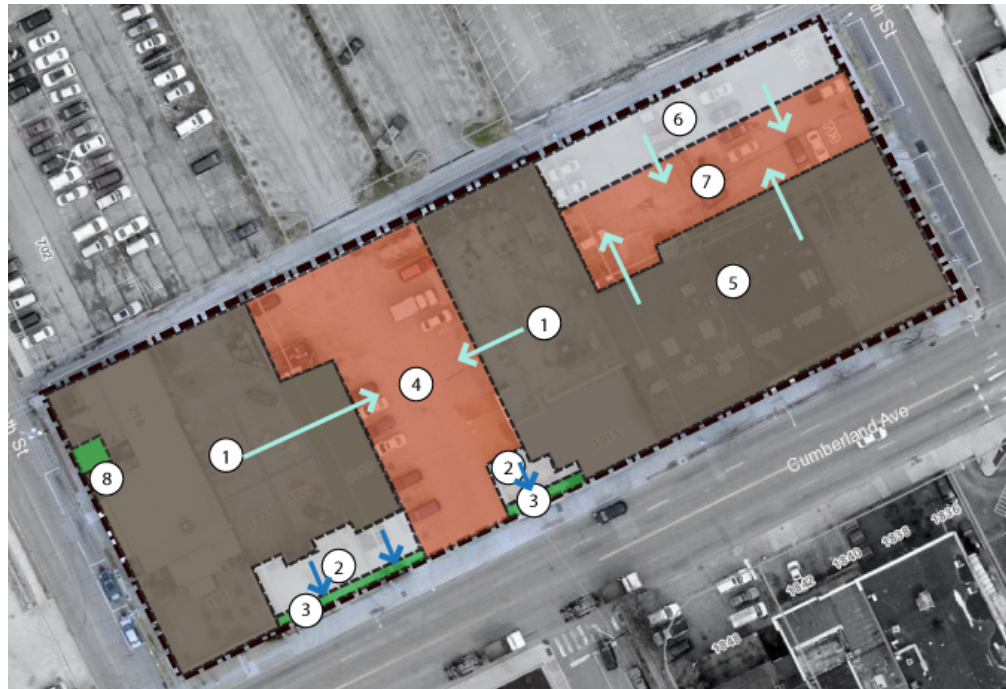
Figure 29: Runoff flow path in the strip mall site
