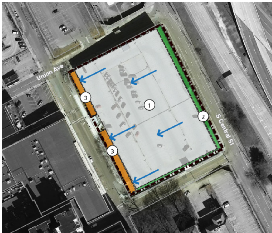
Figure 19: Runoff from rooftop is directed to a bioretention with low vegetation
