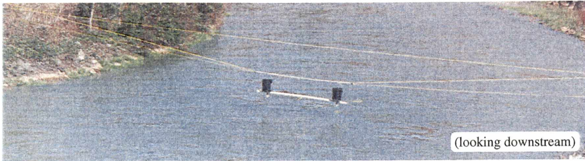
Figure 10. Dye Injection Apparatus at Nottely River Mile 21.0
