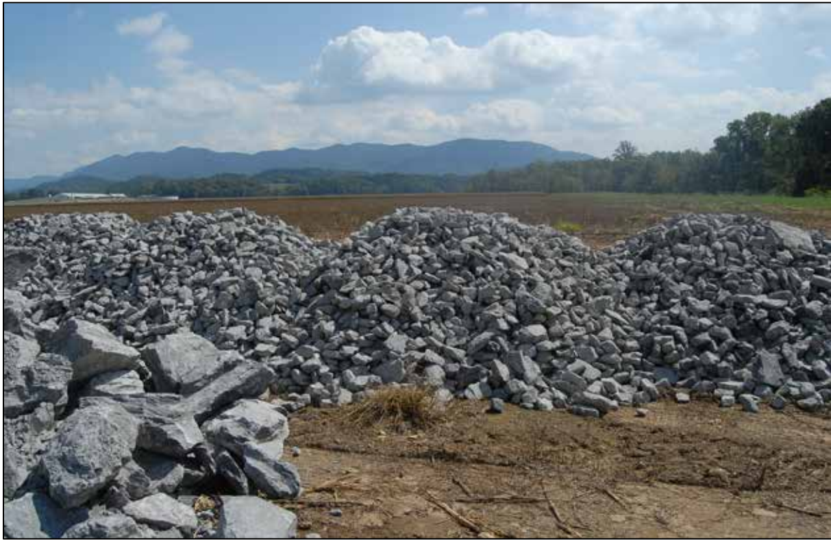
Figure 3.6 –Rock and stone used for filling sinkhole.
