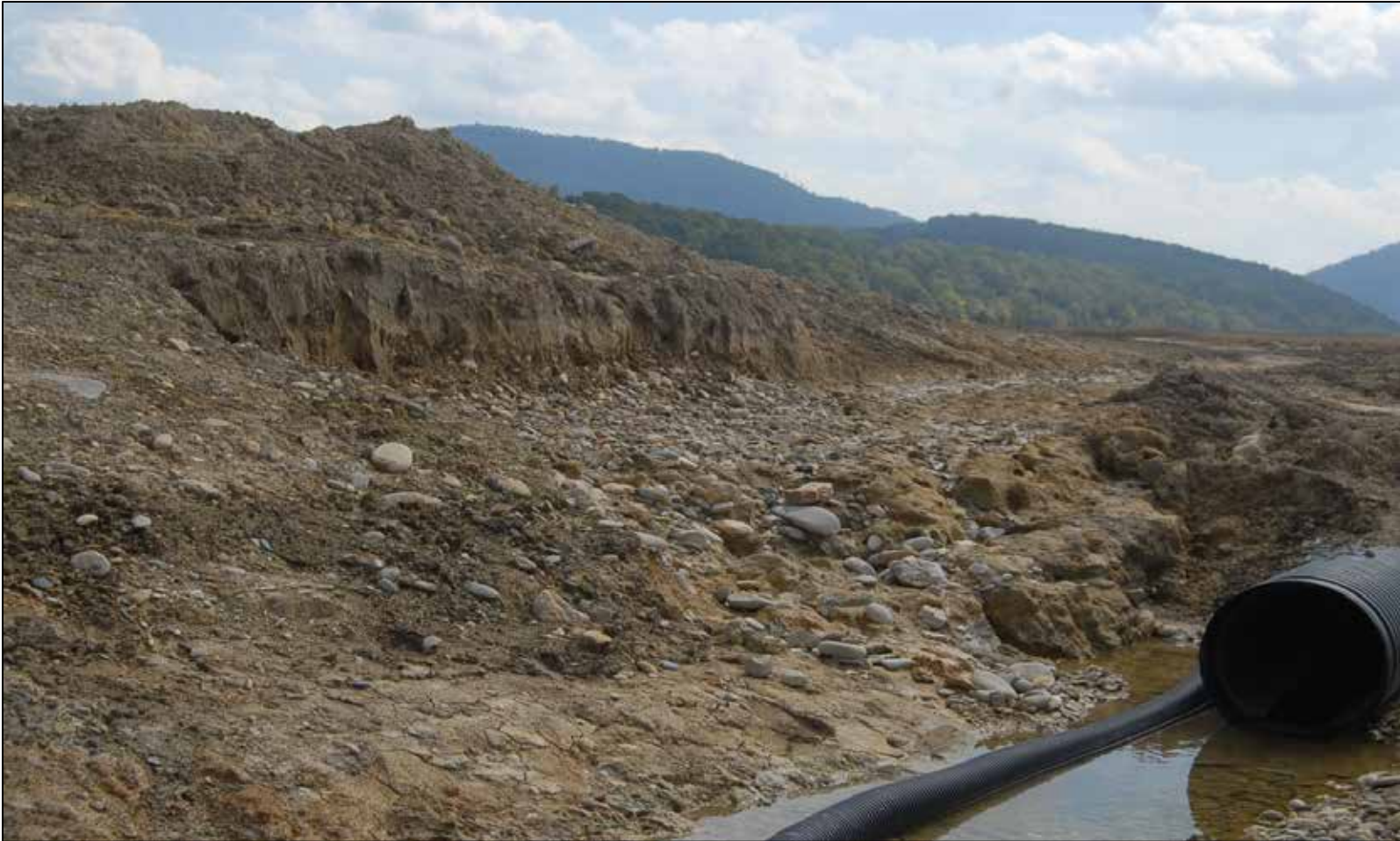
Figure 3.4 – Example of a gravel layer in the floodplain alluvium at LRDF. Note the faint layering in silty sand above the gravel layer.
