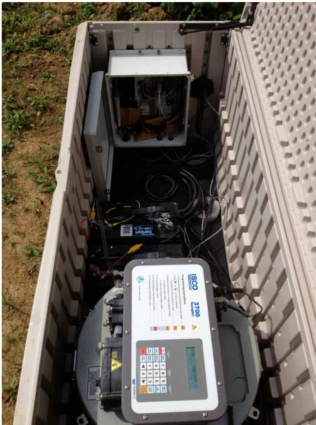
Figure 2.12 ISCO automated sampler unit for the constructed wetland (Ludwig, 2011).
