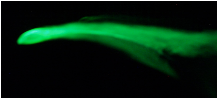
c. Separation Point, x/c=0.60 \pm 0.12 ; \alpha=18 degrees
