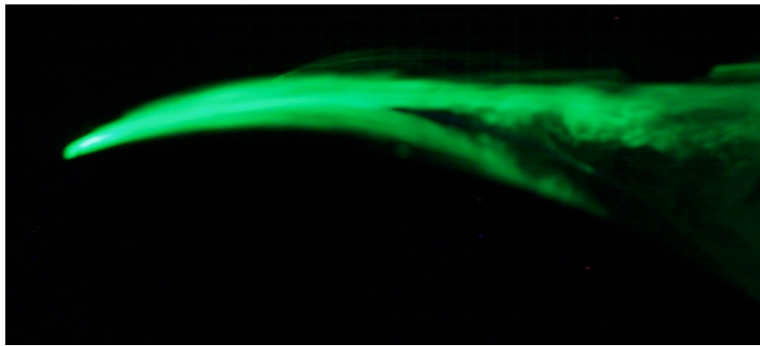
b. Thermocouple Wire at (2,3), Separation Point at x/c=0.42 \pm 0.01
