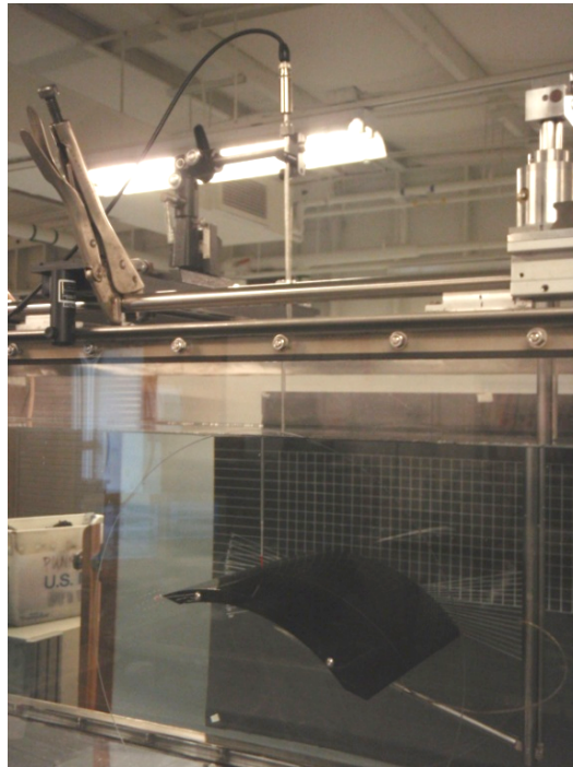
Figure 24. Model Set-up For Hot-Film Velocity Measurements
