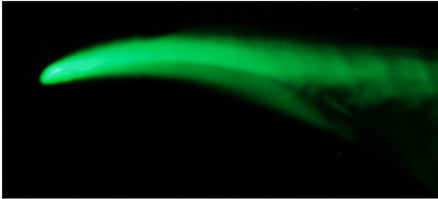
b. Thermocouple Wire at (2,3), Separation Point at x/c=0.59 \pm 0.03
