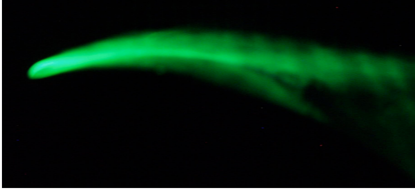
a. Thermocouple Wire at (1,2), Separation Point at x/c=0.62 \pm 0.08
