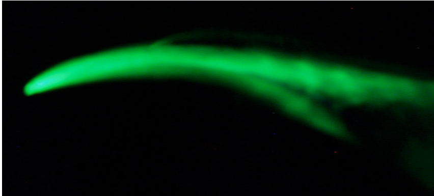
c. Thermocouple Wire at (2,4), Separation Point at x/c = 0.65 \pm 0.08
