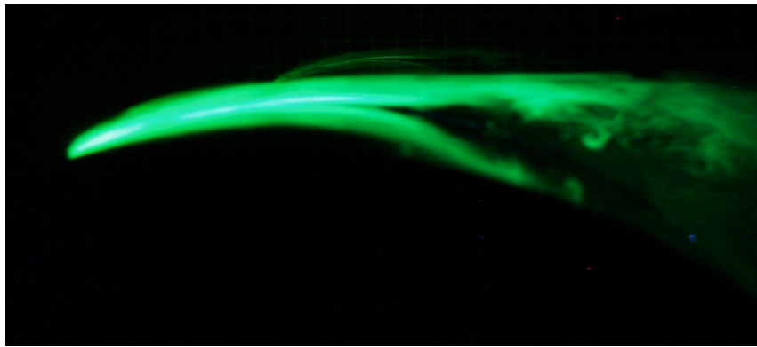
b. Thermocouple Wire at (2,3), Separation Point at x/c=0.39 \pm 0.03
