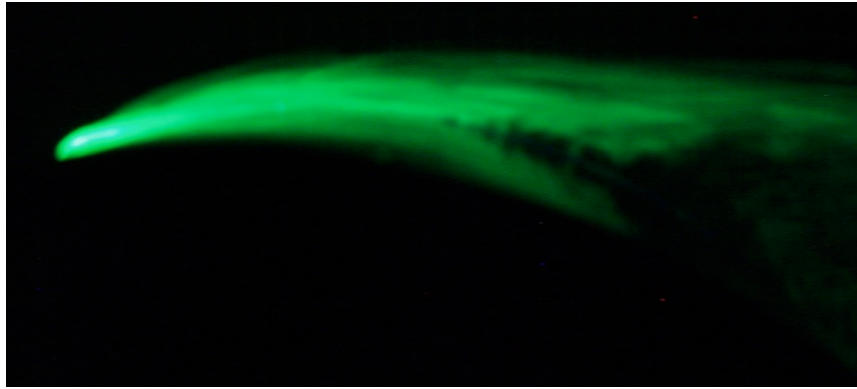
a. Thermocouple Wire at (1,2), Separation Point at x/c=0.55 \pm 0.03
