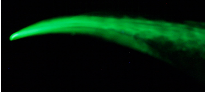
a. Thermocouple Wire at (1,2), Separation Point at x/c = 0.64 \pm 0.06
