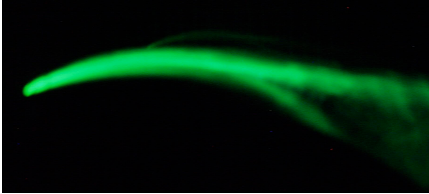
b. Thermocouple Wire at (2,3), Separation Point at x/c = 0.71 \pm 0.05
