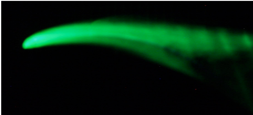
c. Thermocouple Wire at (2,4), Separation Point at x/c=0.54 \pm 0.02
