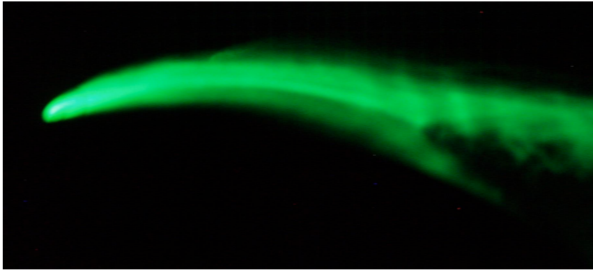
b. Thermocouple Wire at (2,3), Separation Point at x/c=0.69 \pm 0.05
