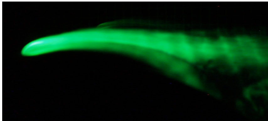
c. Separation Point, x/c=0.69 \pm 0.04 ; \alpha=18 degrees
