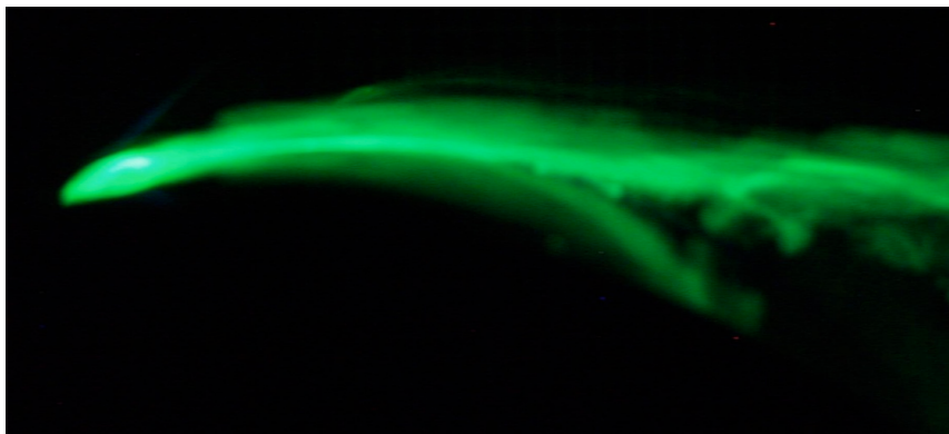
b. Separation Point, x/c=0.50 \pm 0.03 ; \alpha=16 degrees
