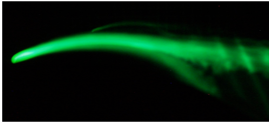
a. Separation Point, x/c=0.67 \pm 0.03 ; \alpha=14 degrees
