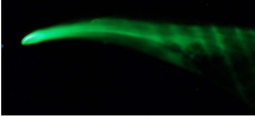
a. Thermocouple Wire at (1,2), Separation Point at x/c=0.60 \pm 0.04
