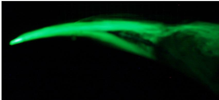
c. Thermocouple Wire at (2,4), Separation Point at x/c=0.43 \pm 0.01
