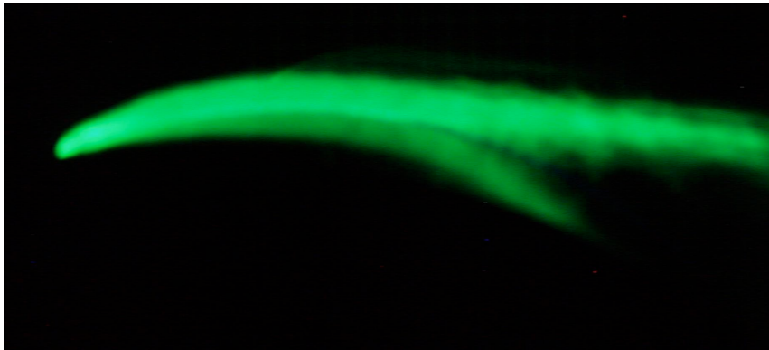
c. Thermocouple Wire at (2,4), Separation Point at x/c=0.60 \pm 0.05
