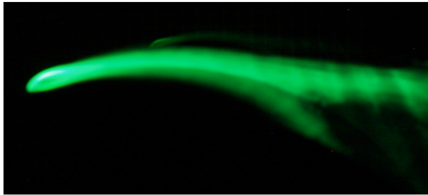
b. Separation Point, x/c=0.65 \pm 0.03 ; \alpha=16 degrees
