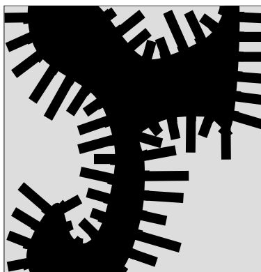
Figure 53 Protruding black molecules forming secondary charge carrier pathways for the black domain.
