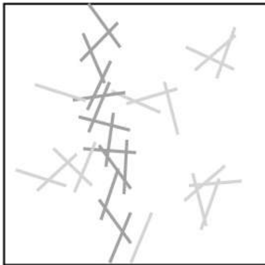
Figure 54 Illustration of percolation of cylindrical rod particles through the bulk. 176
