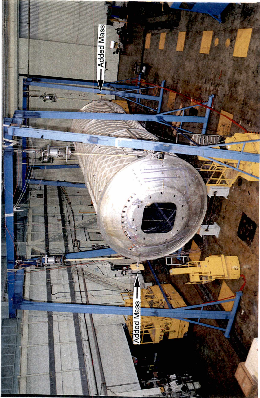
Figure 1.3 Mass Additive Modal Test
