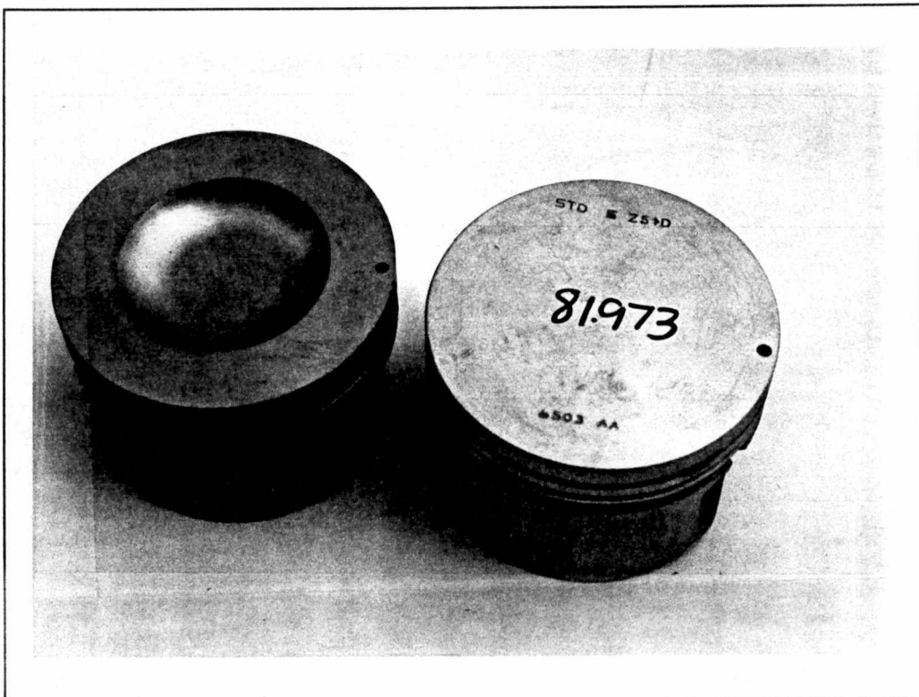
Figure 6: Flathead and stock pistons
