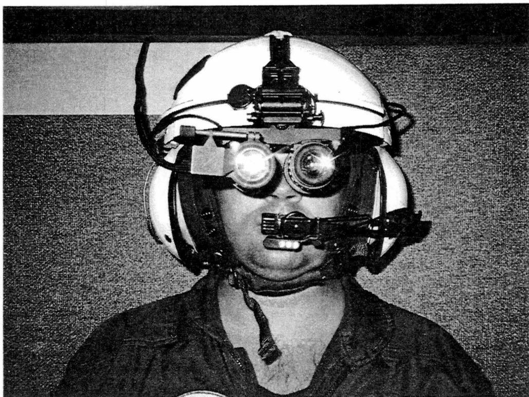
Figure 5. ANVIS-7 Display Driver Unit (DDU) As installed on ANVIS-6 NVGs
