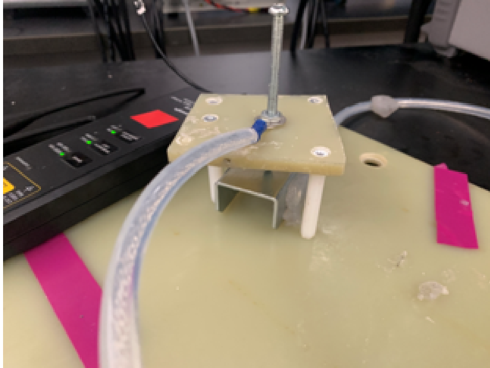
Figure 4.11: Corona Discharge Test subject: high voltage point and grounded plane
