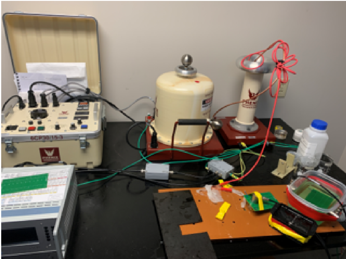
Figure 3.3: Phenix AC Dielectric 30kV Test System
