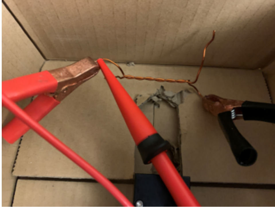
Figure 3.13: Partial Discharge Testing of a twisted pair using photomultiplier tube in a dark environment
