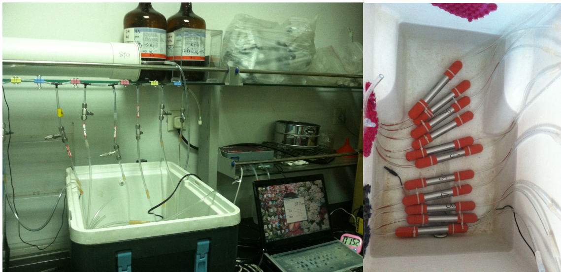
Figure 2: The pictures above depict the soil respiration study setup. The left picture shows the incubation bath, the LiCOR gas analyzer, the cylindrical desiccator, and the flow regulators and tubing apparatus. The right picture shows the individual incubation vessels and the gas-flow tubing that extends from them for measurements and flow regulation.
