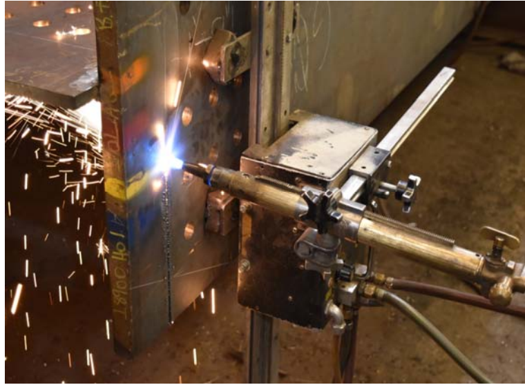
Figure 18: Trimming girder to length. Note that the girder holes would not be present in the traditional method at this point in the process
