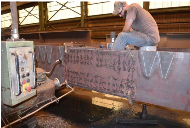
Figure 19: Drilling the web (side view). Note the flange splice plate temporarily secured with clamps.
