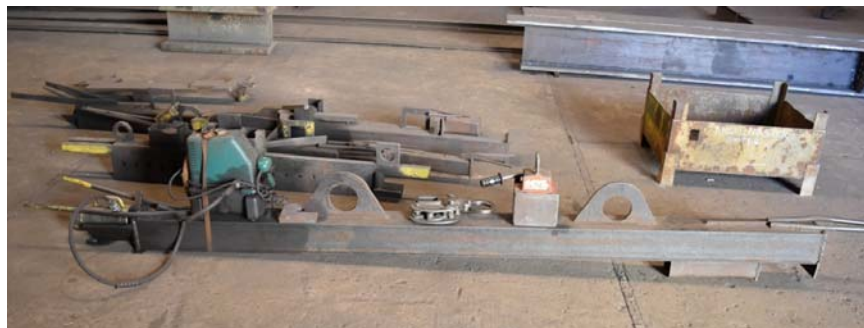
Figure 15: Hydraulic jack used in fitting stiffeners to girders
