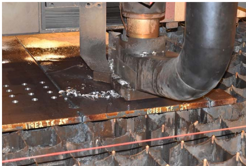
Figure 24: CNC machine drilling a splice plate
