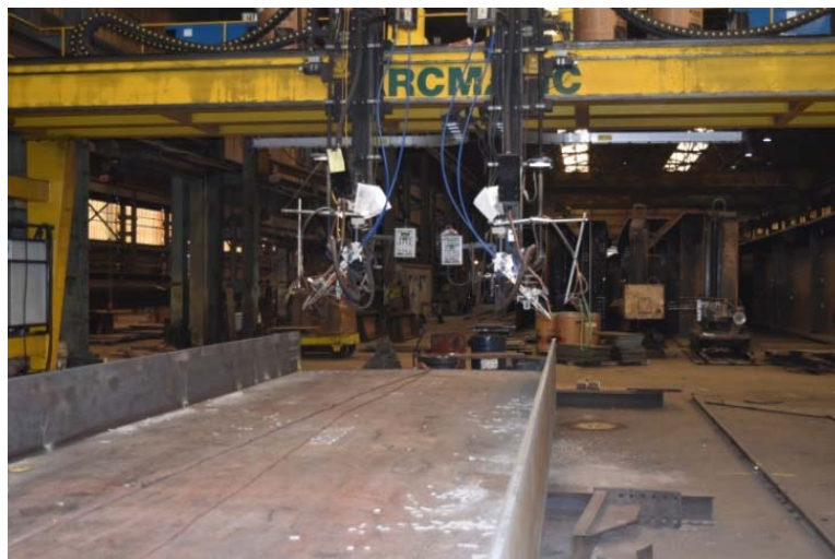
Figure 13: Arcmatic automated welding machine shown prior to welding
