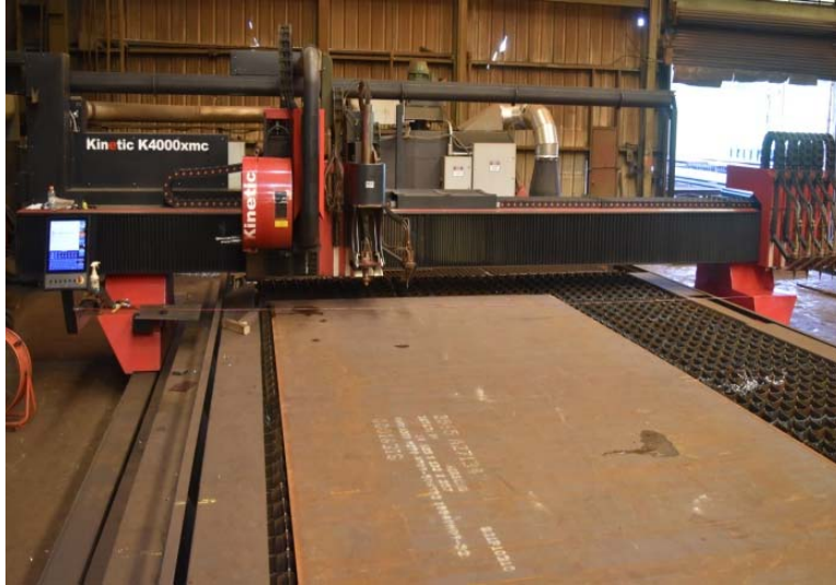
Figure 10: Steel plates on CNC machine
