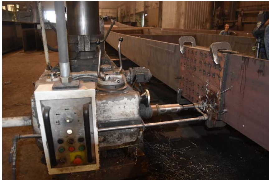
Figure 21: Match drilling flange plate
