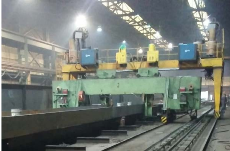
Figure 12: Squeezer machine used to temporarily hold girder plates together in preparation for welding
