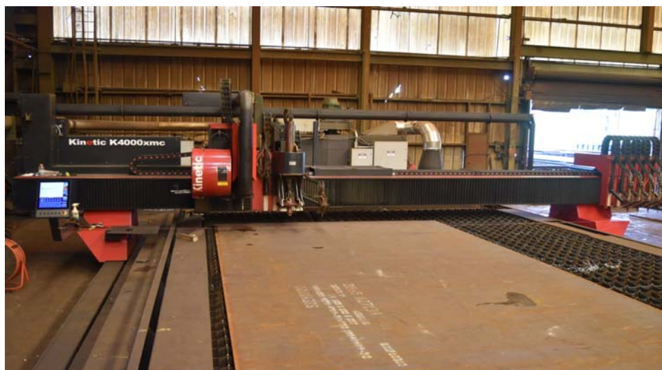
Figure 1: CNC cutting and drilling equipment
