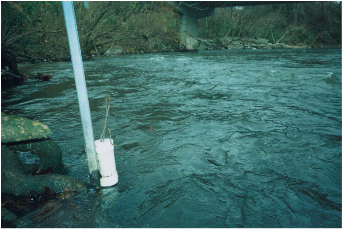
Figure 6. Retrofitted bottle attached to the sampler
