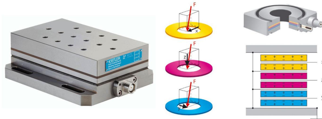
Figure 2.9: Kistler 9257B (left) and the diagram of the piezoelectric crystals arrangement (right) [13].
