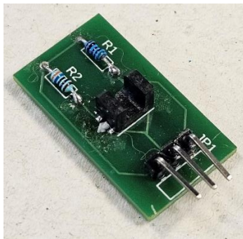
Figure 3.1: Image of ROHM RPI-0352E sensor (left) and corresponding circuit diagram (right)
