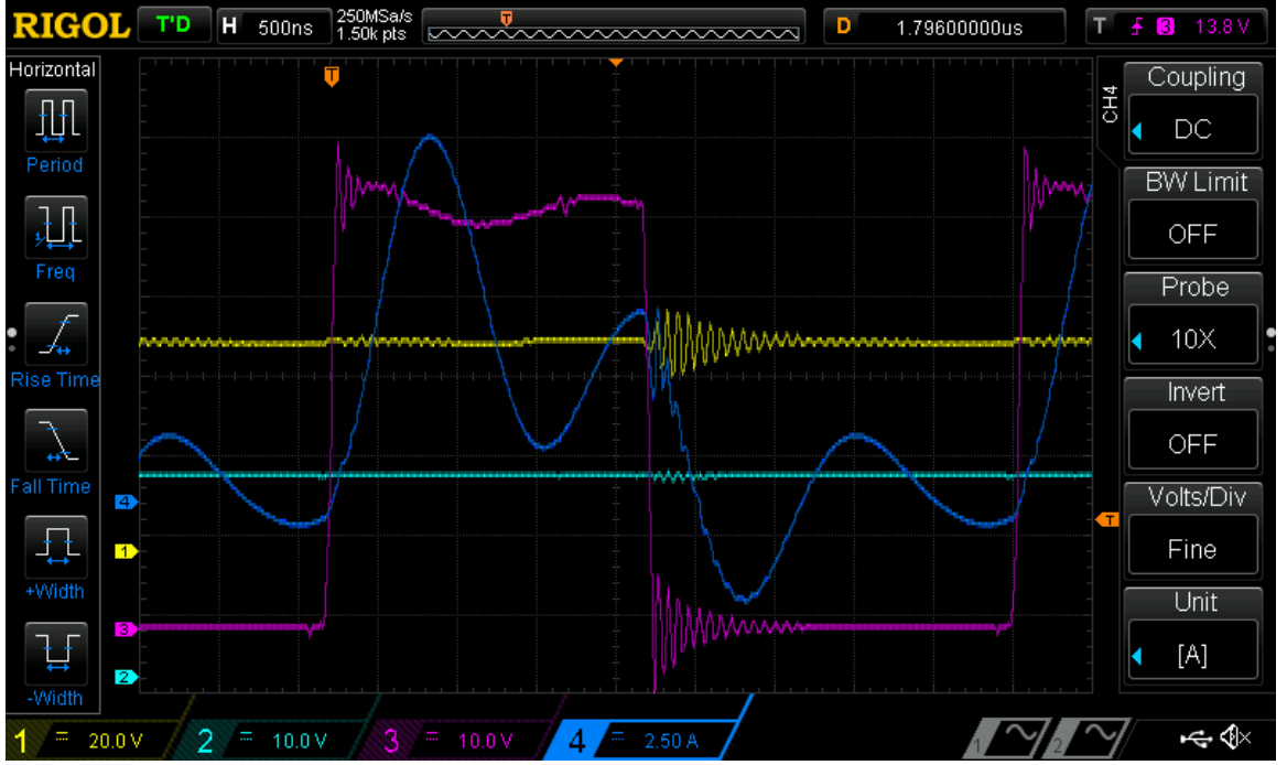
Figure 4.7: High Side MOSFET Current (after decoupling cap): V_{sw} (Pink), I_{dH} (Blue), V_{batt} (Teal), V_{out} (Yellow)
