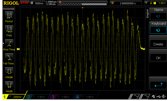
Figure 2.4: P = 2 * 23\text{Hz} = 46 poles
