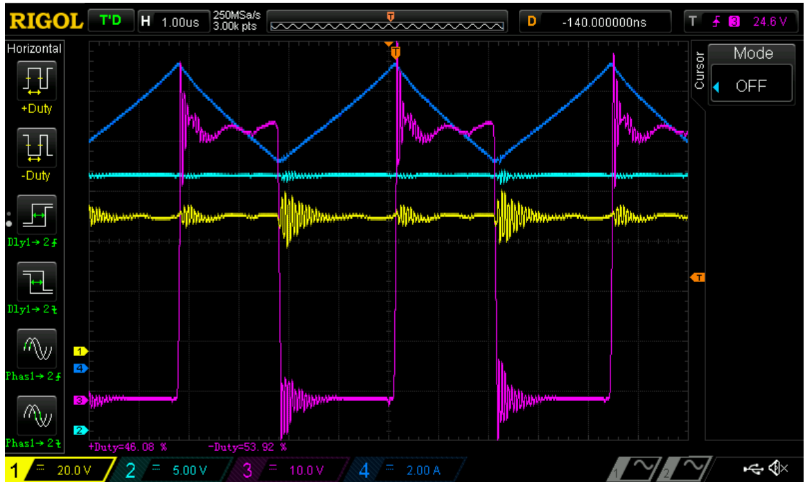
Figure 4.5: Full Power: V_{sw} (Pink), I_L (Blue), V_{batt} (Teal), V_{out} (Yellow)
