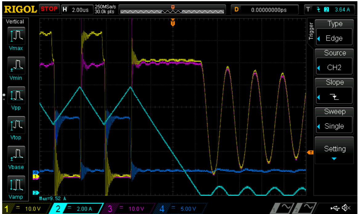
Figure 5.15: Failure from Sense Resistor Parasitics with I_{ind} (light blue), V_{gsL} (dark blue), V_{goH} (yellow), V_{sw} (pink)
