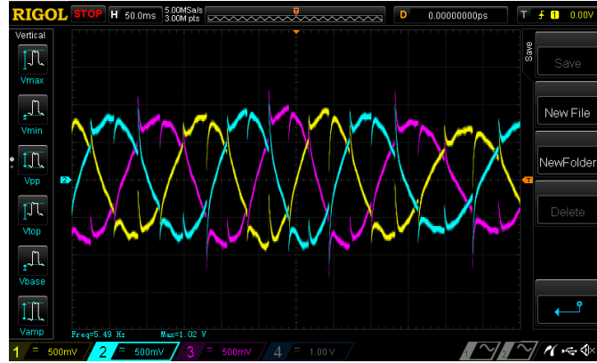
Figure 2.1: \lambda_m = 1.02V/(2\pi * 5.49Hz) = 29.6 \text{ mWb}
