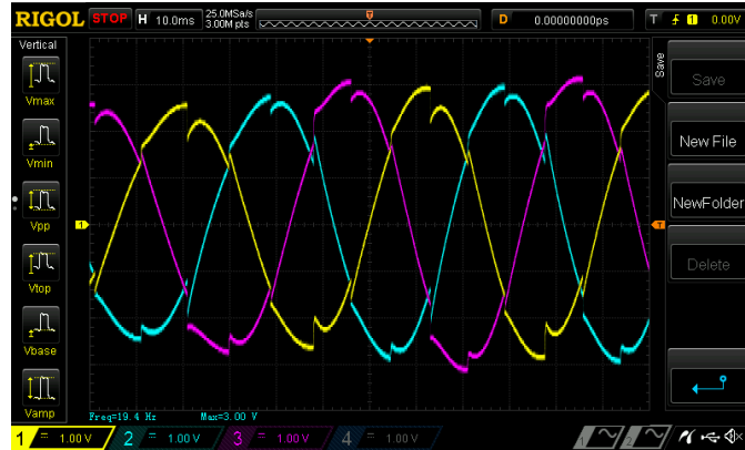
Figure 2.3: \lambda_m = 3V/(2\pi * 19.4Hz) = 24.6 \text{ mWb}
