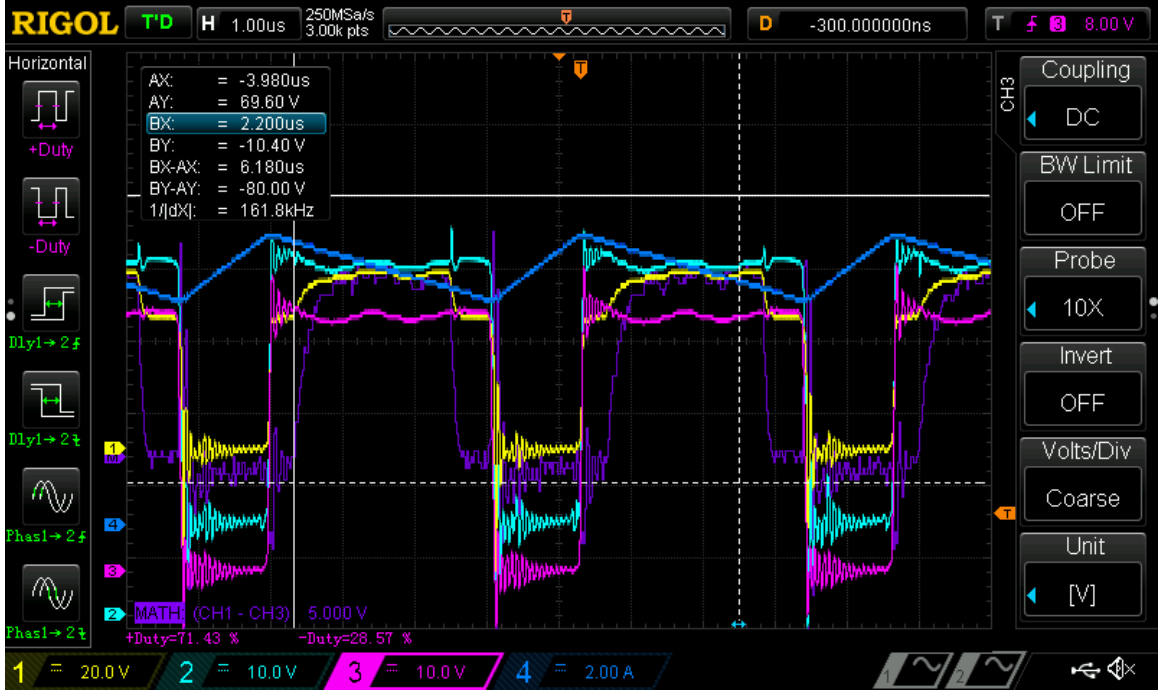
Figure 4.12: Efficiency Sweep at 34 V output: V_{sw} (Pink), I_L (Blue), V_{hb} (Teal), V_{ho} (Yellow), V_{gsH} (Purple)
