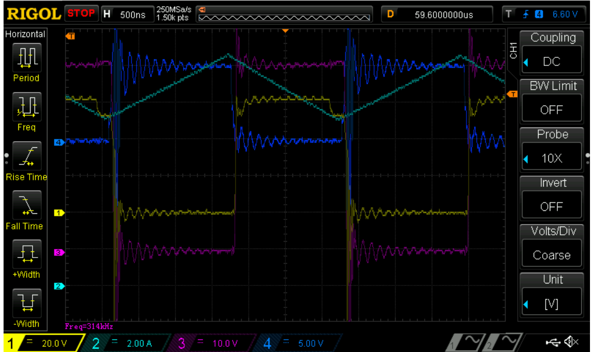
Figure 8.2: 250 W Boost Converter after PCB assembly with I_{ind} (light blue), V_{gsL} (dark blue), V_{goH} (yellow), V_{sw} (pink)
