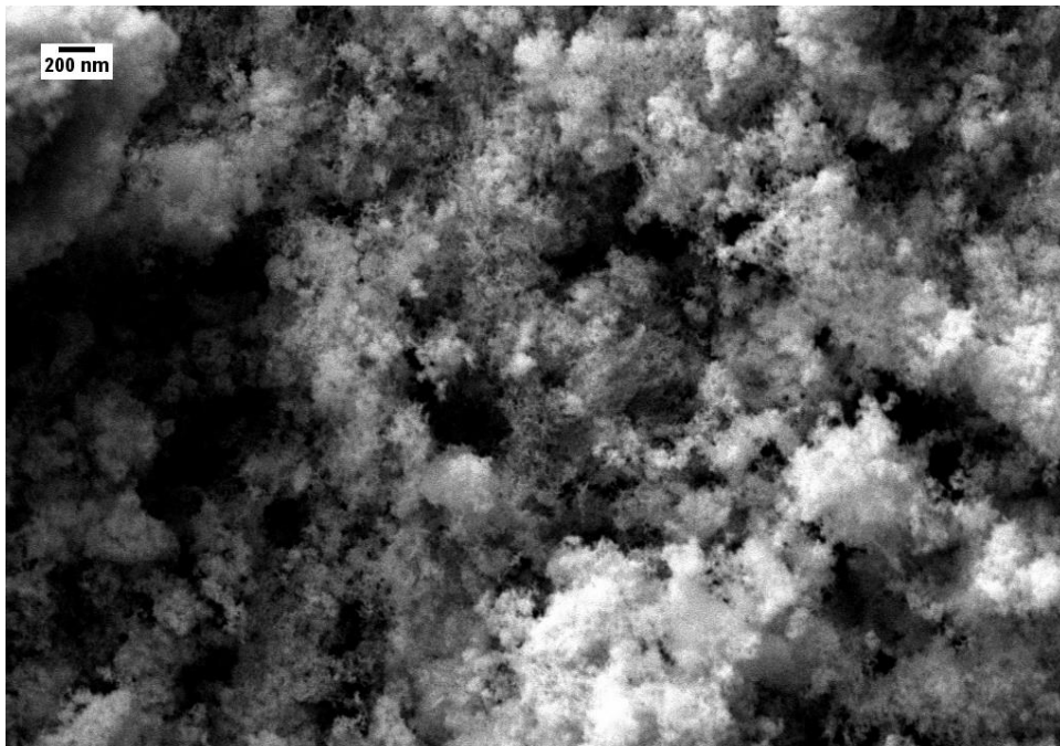
Figure 43: Closer SEM image of boron carbide on 10 \Omega -cm silicon. This image suggests a polycrystalline or amorphous film, rather than single-crystalline.
