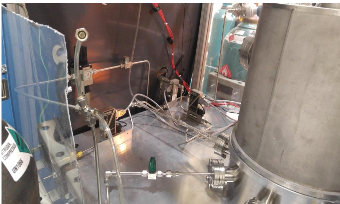
Figure 29: Gas lines before getting into the chamber (with the nitrogen disconnected from changing tanks).
