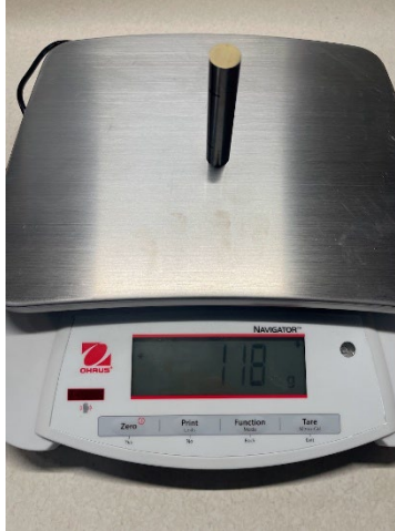
Figure 4-13. The mass of the tool shank was measured and used to calculate the carbide shank density.
