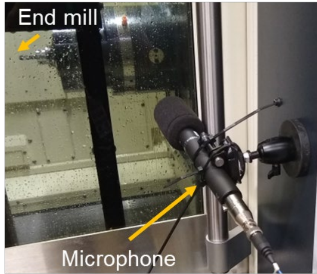
Figure 4-49. For each stability test, the cutting sound was recorded and was stability determined by frequency content.
