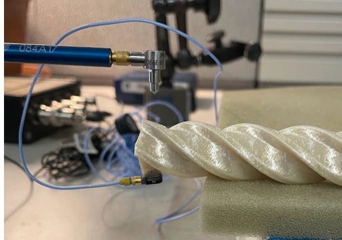
Figure 4-6. Free-free impact testing of an additively manufactured tool flute geometry.
