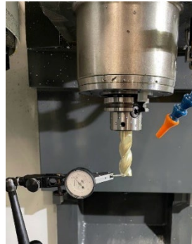
Figure 4-46. Runout of the tool was measured using a dial indicator.
