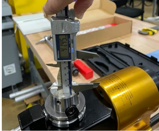
Figure 4-33. Calipers were used to measure the stickout length of each carbide rod and tool.
