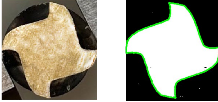
Figure 4-22. (Left) An image was taken of the tool cross section at the sectioned plane. (Right) The photo was converted to a binary image, and the points around the profile were identified using an image tracing function in MATLAB.
