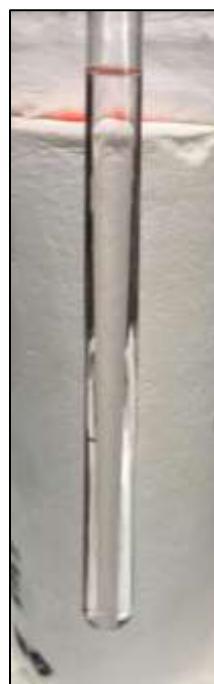
Figure 2.2.1 Solid KCl/MgCl 2 mixtures loaded in silica tubes inside glovebox (top). Molten distilled MgCl 2 at 800°C, 150 grams (bottom left). Molten distilled MgCl 2 at 800°C, 10 grams (bottom right).
