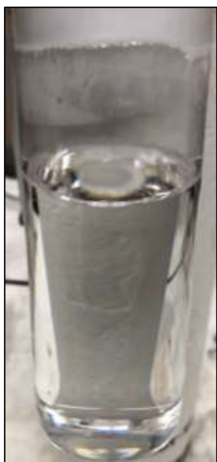
Figure 2.2.1 Solid KCl/MgCl 2 mixtures loaded in silica tubes inside glovebox (top). Molten distilled MgCl 2 at 800°C, 150 grams (bottom left). Molten distilled MgCl 2 at 800°C, 10 grams (bottom right).
