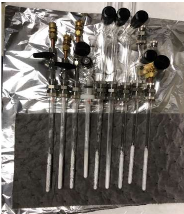
Figure 2.1.1 Schematic representation of vacuum valve connection to small diameter silica tube (top). Pictorial representation of vacuum valve connection to small diameter silica tube (bottom).
