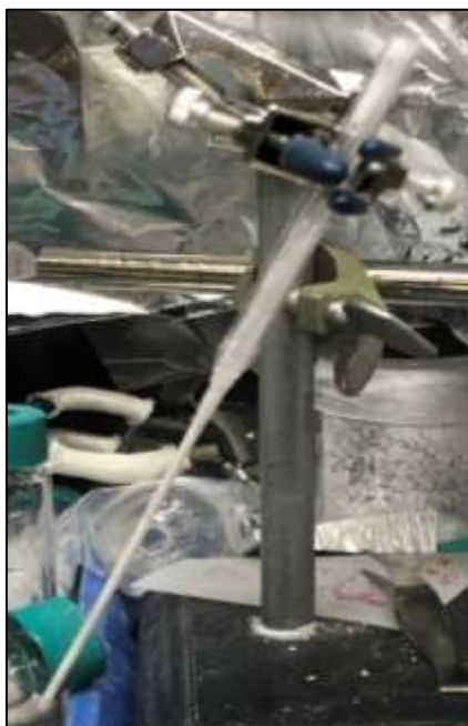
Figure 2.5.1. Pictorial representation of 2.0 mm X-ray capillary purchased from Charles-Supper with added extension loaded with \text{MgCl}_2 .
