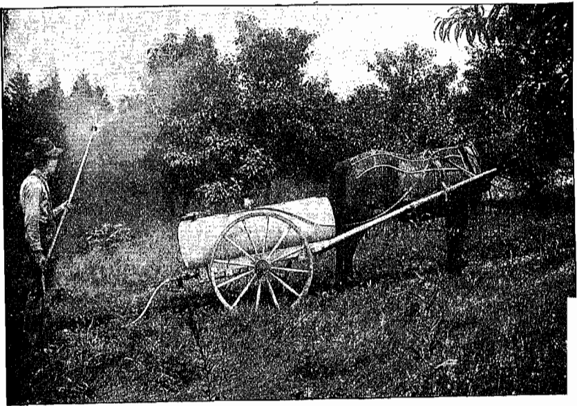
FIG. 20. COMPRESSED AIR SPRAYER; EFFICIENCY WITH LITTLE WEIGHT
