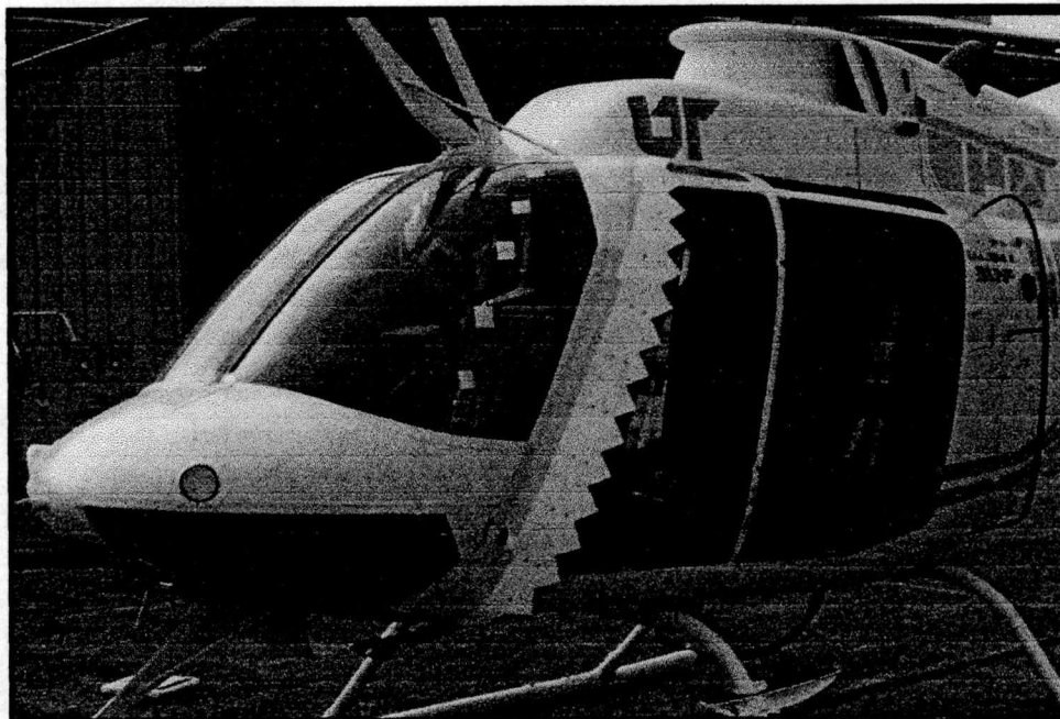
Figure 6.1: Installed Sawtooth Diverter
