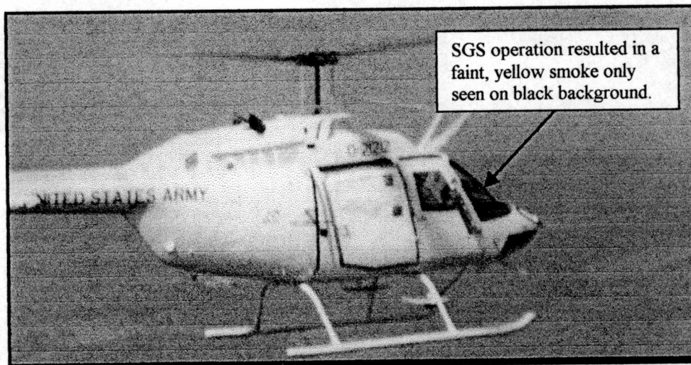
Figure 7.5: SGS Operation in Flight (Yellow Canisters)
