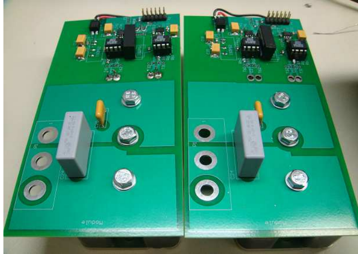
Figure 7-11. Developed phase-leg module with IGBTs (Version-1)
