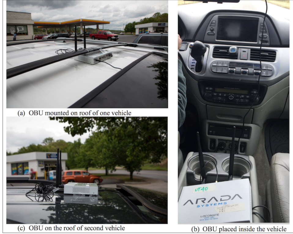
Figure 2.2: Placements of OBUs (rooftop and inside)
