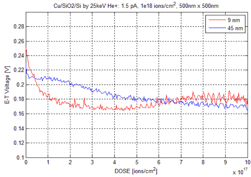
Figure 3.35. Responses collected for two (2) different copper top layer thicknesses when etched by helium.
