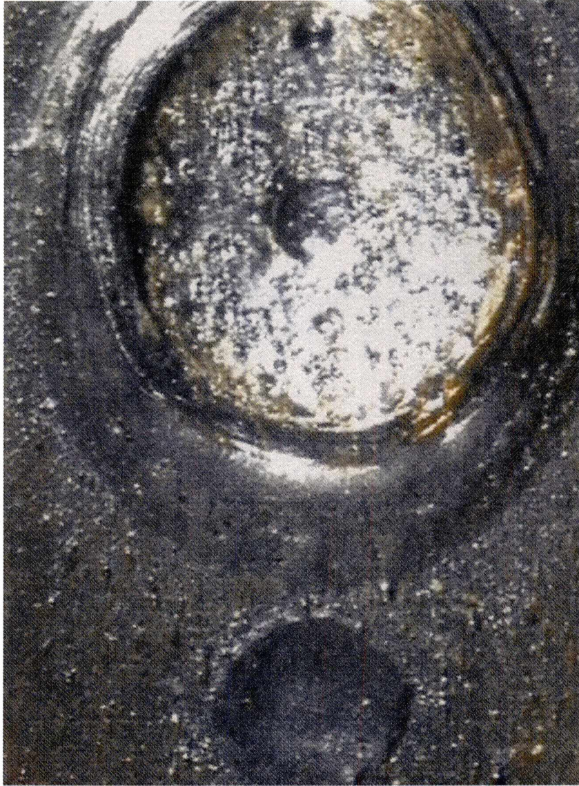
Figure 12. Improper Alignment of Plasma Torch with Laser.
