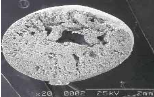
Figure 1-2 Cross section of Bio-Sep® bead.
