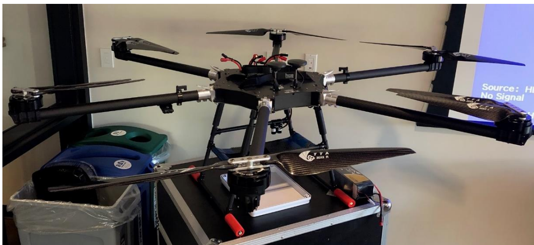
Figure A.29. HL-6 Aircraft with Flexible Carbon Fiber Platform Constructed between Leg Spreaders
