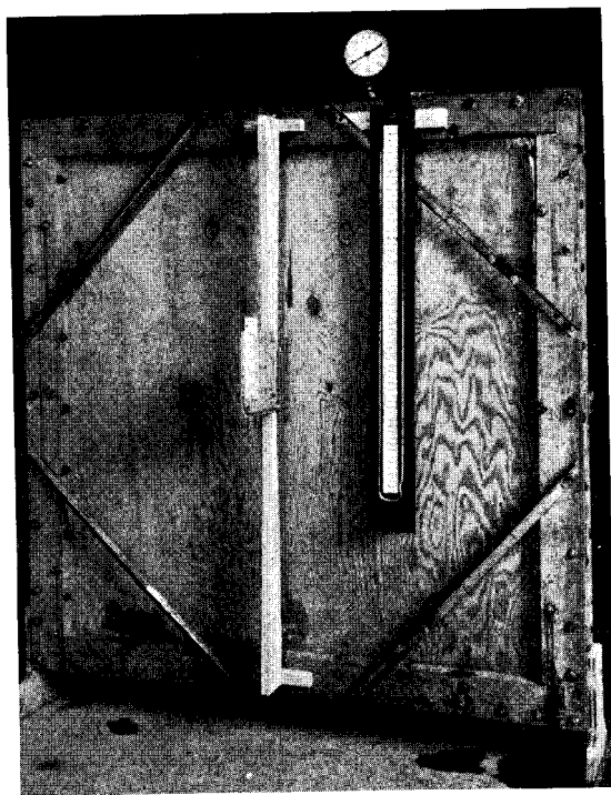
Fig. 6—Plywood panels under test, showing pressure and deflection gages.
